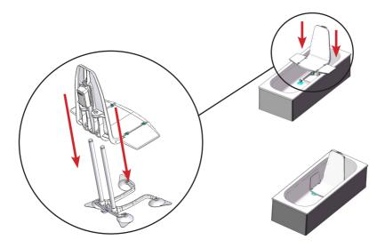
The actuator assembly should be housed securely; to house the actuator assembly, lie it against the backrest, slotting the shaft through the actuator guide at the bottom of the seat. Then place the actuator shaft within the base actuator socket the actuator is held in place by gravity and should be securely housed in the slot.
